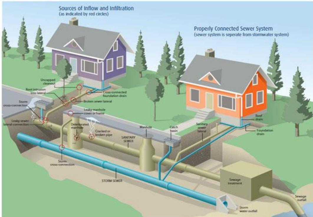
**Separated Sewer Systems** are piping systems with separate storm and sanitary sewer pipes. The purpose of having separate pipes is to convey only sanitary or storm water in the respective pipes. By accomplishing this level of separation, capacity issues in the sanitary sewer during storm events are eliminated and will perform similarly as during dry days.
