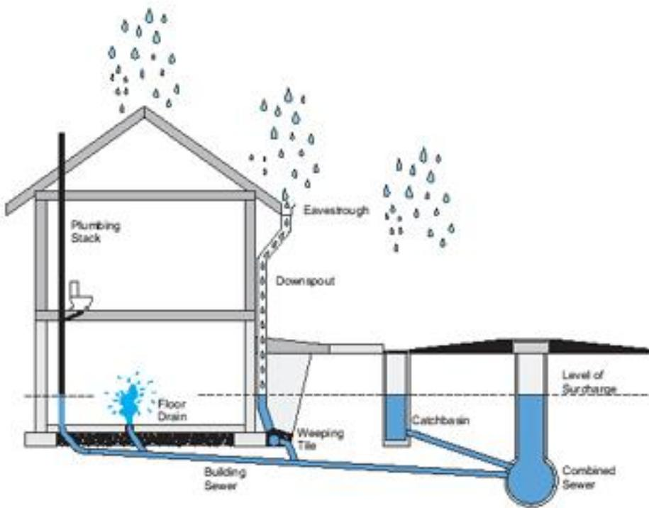
**Combined Sewer Systems** are piping systems that share one pipe for both storm and sanitary sewer flows. Combined sewer systems are common in older cities constructed prior to the Clean Water Act of 1972. Combined systems are typically supplemented with regulated overflows to relieve the sewer during heavy rain events. MDC has been actively working over the past two decades to reduce the occurrences and volume of overflows through its Clean Water Project.
